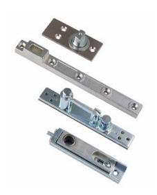
The Briton 7500 Series is designed to accomodate architectural and oversized doors. Pivot sets provide a seamless way of hanging doors, with the option to be swinging in either direction. It suits doors with a minimum thickness of 40mm, and a width up to 1400mm.
